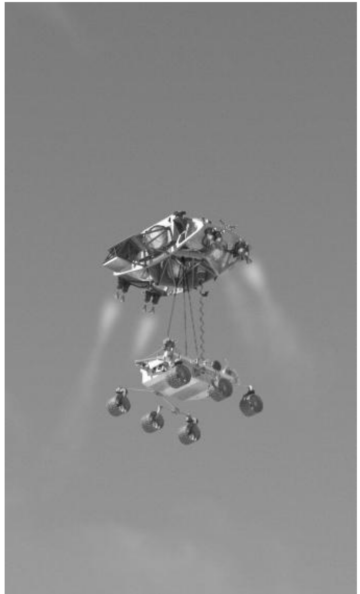
The Curiosity rover will use an innovative "sky crane" system to land on Mars. A rocket-powered carrier will lower the rover to the surface, as the craft is too big to use the airbag system previous rovers have used (NASA/JPL)
