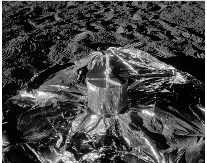
An Apollo Passive Seismic Experiment deployed on the lunar surface (NASA)
